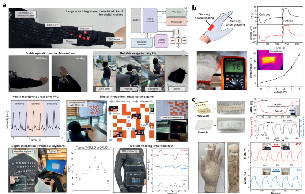
Fig. 1. Conductive fibers and their applications in wearable technology, human-machine interfacing and soft electronics. (a) Thermally drawn liquid metal fibers and their applications in everyday activities, health monitoring and wearable circuitry. Adapted under the terms of CC-BY 4.0 license from [11]. (b) PEDOT:PSS based conductive fibers and their applications in wearable technology, as heat transducers embedded in to a glove. Adapted under the terms of CC-BY 4.0 license from [16]. (c) Carbon-composite polymer fibers as sewable or knittable temperature sensors, integrated into fabrics and commercial gloves. Adapted under the terms of CC-BY 4.0 license from [31].
