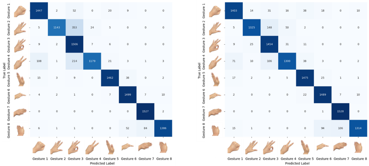
Fig. 11. Classification performance of the proposed model, illustrating confusion matrices for two individual subjects.
